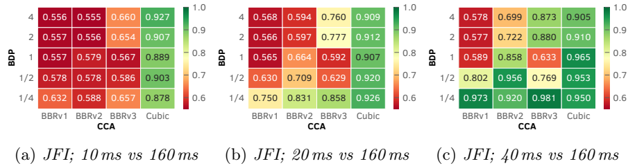
Fig. 14: Average Jain's fairness index ( JFI ); short RTT flows (10 ms, 20 ms, 40 ms) start first, then 15 s later the 160 ms flow starts.
