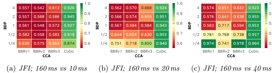
Fig. 11: Average Jain's fairness index (JFI); 160 ms flow starts first, then 15 s later the (10 ms, 20 ms, 40 ms) flow starts.
